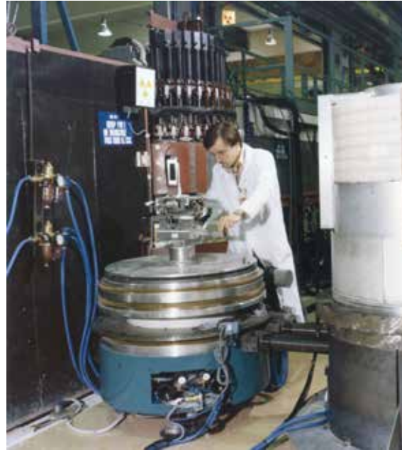
Building IN12 - First new-generation 3-axis instrument.
