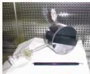
The helium-3 cell used as a source of polarised neutrons
