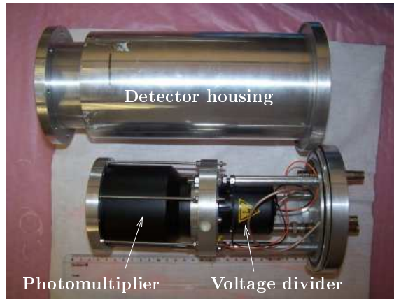
Figure 10.2: Set-up of the scintillator detectors.
