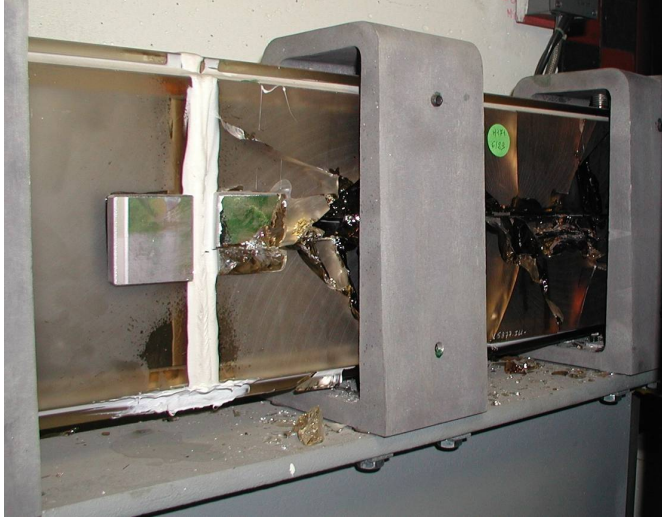
(a) H17 guide after implosion
