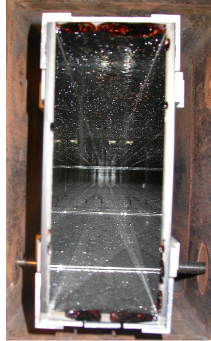
(b) H113 guide, peeling of the mirrors
