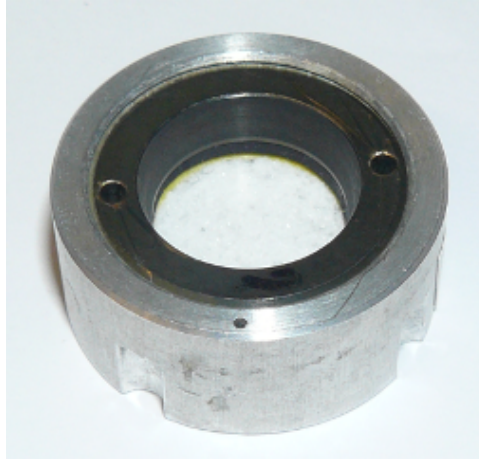
Figure 4.16: D11 cell filled with crushed glass
