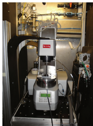
Figure 3.27 – In situ Rheo-reflectometry on FIGARO from reference [138]
