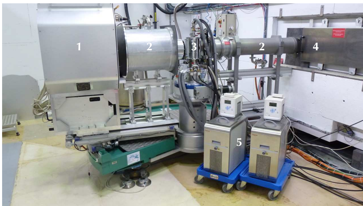
Figure 3.8 : Side view of D16 with the major components highlighted. (1) Detector, (2) evacuated tubes, (3) sample position, (4) neutron guide and monochromator position, (5) water baths for temperature control.
