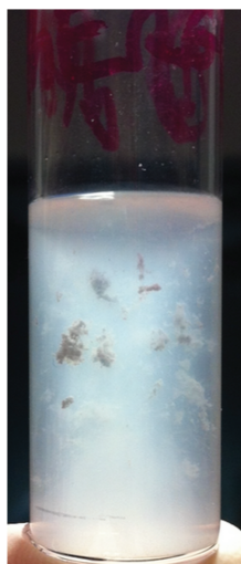
Figure 4.9 : Representative sample after sonication showing the turbidity of all the P. pastoris lipid-containing samples prepared with high calcium presence (100mM NaCl and 20mM CaCl 2 ). The same samples prepared in 100mM NaCl only or no salt at all (plain water) were perfectly clear after sonication.
