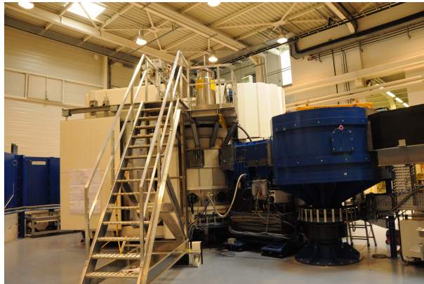
Figure 4.12: Photograph of the backscattering spectrometer IN16B at the Institut Laue-Langevin. (Courtesy Serge Claisse, ILL)
