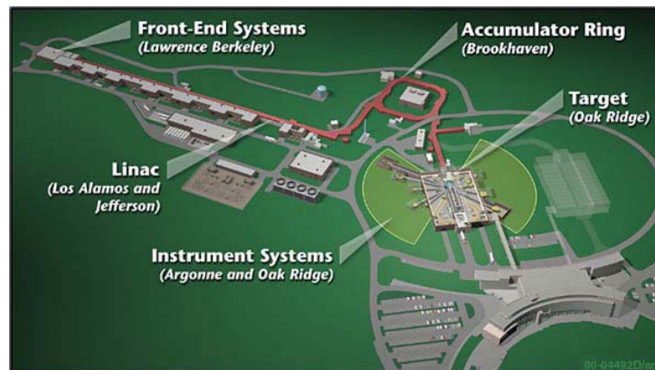
Figure 4.11: Three-dimensional scheme of the Spallation Neutron Source facility. Ions produced at the front-end system are accelerated in the linac, at the end of which protons are produced and stored in the accumulator ring. When the a proton bunch is ready, it is directed to the target, where neutrons are produced by spallation and delivered to the instruments. Figure created by John Jordan, Oak Ridge National Laboratory [190].
