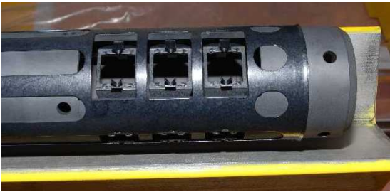
Figure 2.4: Top view of the trolley. The three mounting positions for target containers are visible. The diameter of the trolley is about 15 cm.
