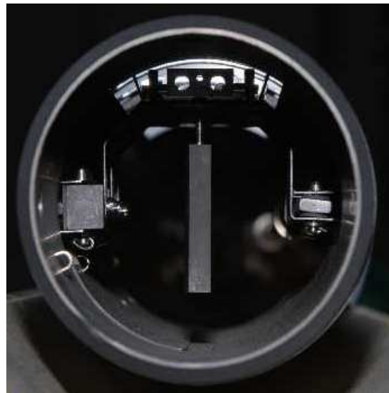
Figure 2.5: Face view of the trolley with a target container mounted. The mechanism for rotating the target containers while being in the beam tube is visible at the sides.
