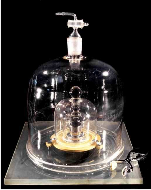
Figure 1.3: The kilogram prototype. Hosted at BIPM under 3 glass shields in standard air. Photograph from BIPM.
