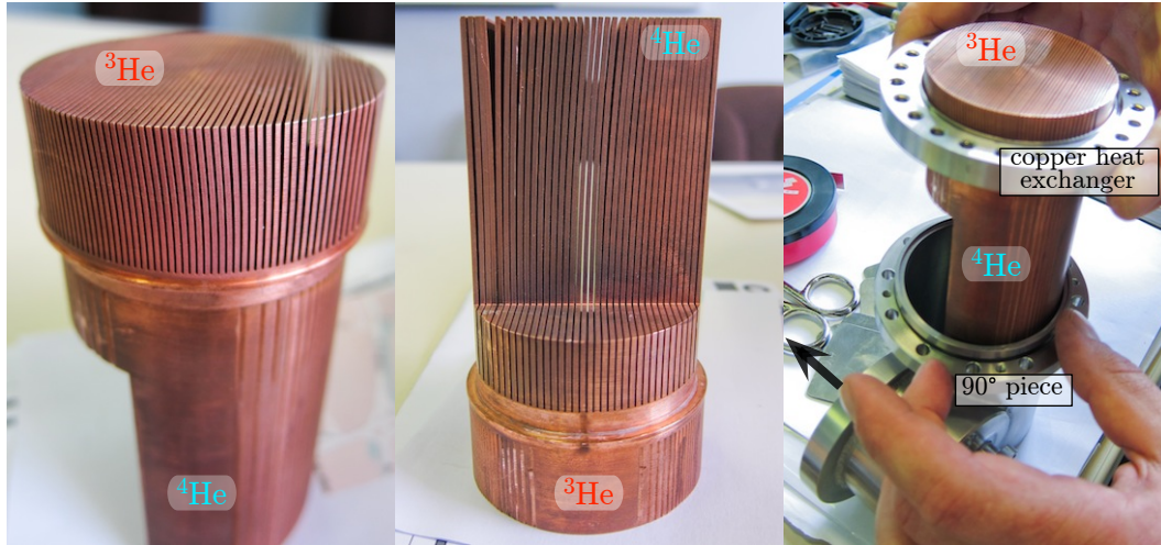
Figure 2.12: The “hair comb” copper heat exchanger used in SUN2. Labels indicate the ends used for the ^3\text{He} and ^4\text{He} . On the far right, the position of the 90^\circ piece below the heat exchanger is shown. The arrow \leftarrow indicates the direction of the horizontal transfer tube.
