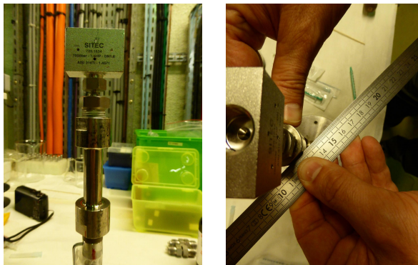
Figure 4-5: On the left: the body of the cross fitting is mounted on the cell via the high-pressure capillary that seals the cell. On the right: the orientation between the fitting and the cell is checked, using as a reference one of the flat surfaces at the end of the cell.
