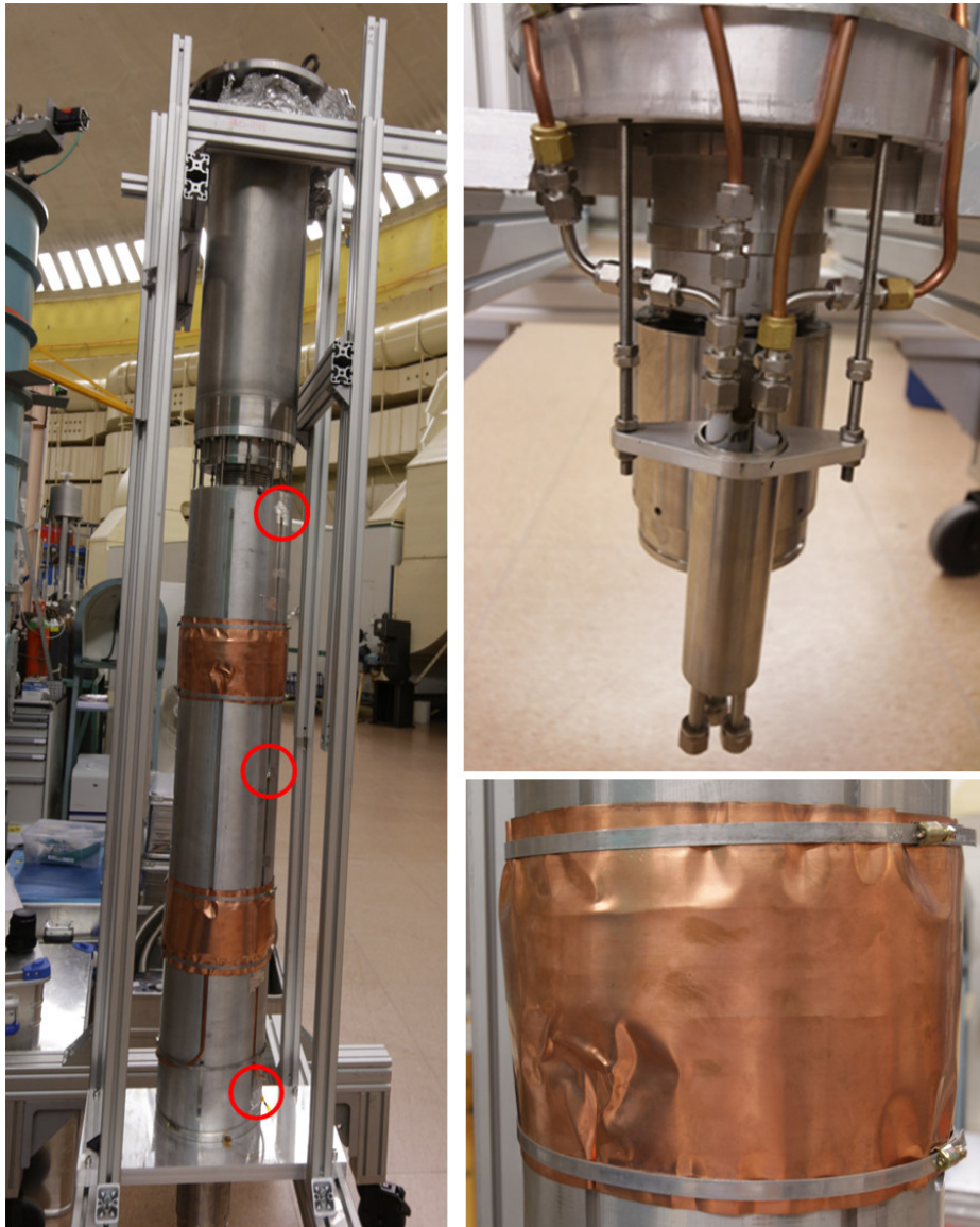
Figure 2.3.: The PMS before its installation in the cryostat. We equipped the PMS with two independent copper spirals for the LN 2 cooling. We have only three feedthroughs for the two spirals as their exit is short-cut (right hand side, top). The red circles show the positions of the PT100 temperature sensors we use as feedback for our P-loop temperature control. The spirals were held in place by the two copper sheets we wrapped around the PMS and fixed by several collars (bottom right). If we had mounted the collars directly on the spirals their fixing screws would have stuck out too far and touched the cryostat's inner bore.
