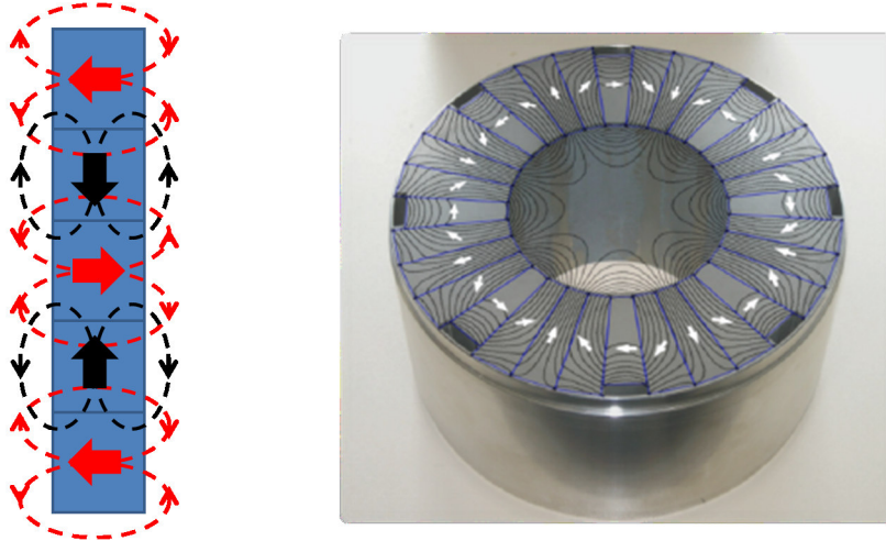
Figure 2.2.: The left hand side shows a schematic illustration of a Halbach-type array. The array consists of single permanent magnet pieces with different magnetisation directions. The particular pattern is chosen in such a way that the field lines of the single pieces will reinforce each other on one side of the magnets while they are canceling each other out on the other side. The picture on the right hand side shows one of our permanent magnet modules. It consists of a total of 32 single magnets. The magnetisation direction of the single magnets is indicated by the white arrows while the gray lines denote course of the magnetic field lines as they have been obtained from some FEMM simulations. Compared to the schematic the pattern contains additional transition pieces as the magnetisation direction from one piece to another only changes by 45^\circ . Therefore the 32 pieces add up to form 8 virtual magnetic poles resulting in the eponymus octupole field inside the bore.
