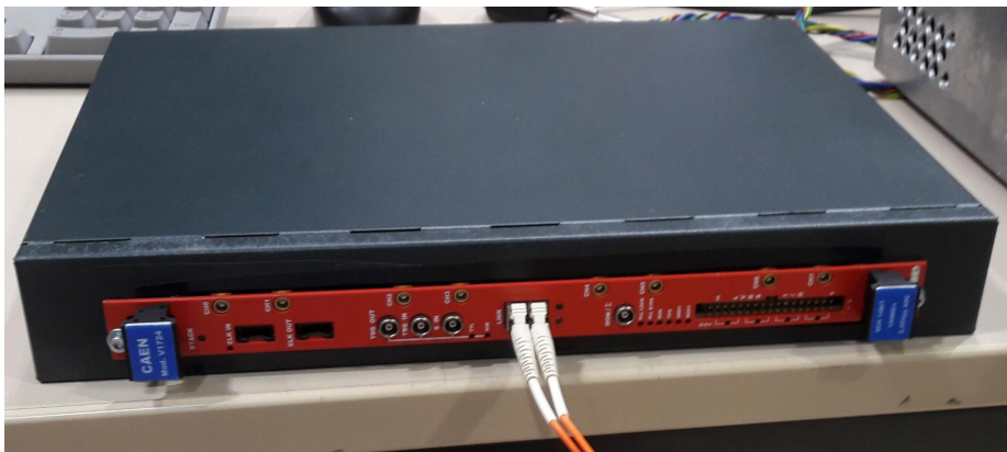
Figure 5.14. The V1724 ADC card in its dedicated box. This VME card can be controlled using only its optical link (front connector) but requires an external power supply and all its VME flags need to be set at their ground level. This is done through the use of a specifically built power supply. Both the ADC box and its power supply are cooled by several fans and are installed in the plexiglass box regrouping all the detector electronics sitting at HV.
