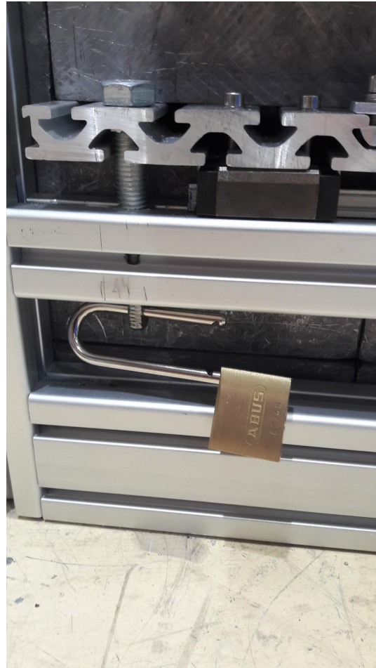
Figure C.3. Zoom on the lock of the lead castle. If the bolt is installed then the castle door cannot open at all.
