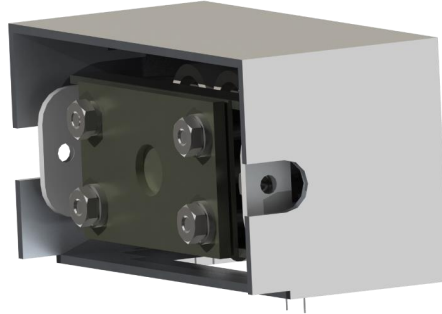
Figure 7.3. Aluminum thermal radiation screen for the crystal holder. Only a few mechanical adjustments are required on the CALIPSO outer box to install this upgrade.
