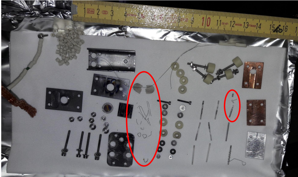
Figure 7.7. Picture of the damaged parts (in red) of the crystal holder: the high-thermal conductivity ceramic (top left), the hot cathode filament (bottom left) and one of the alumina tubes (right).
