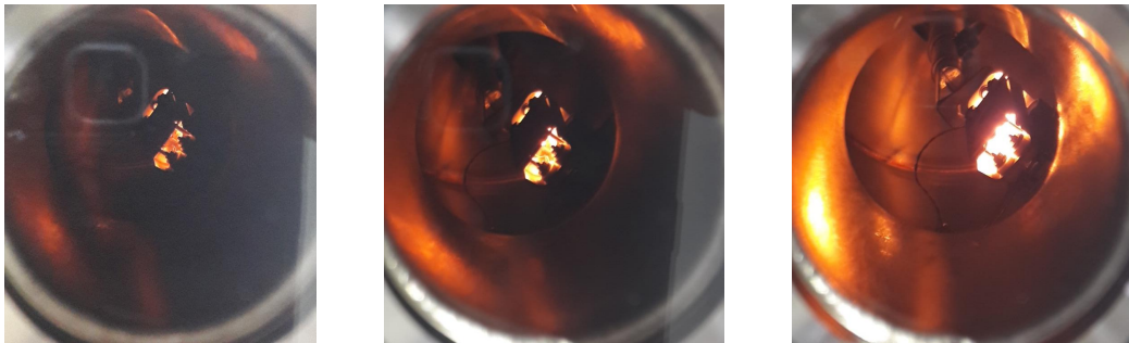
Figure 7.5. Pictures of the inside of the cross source of aSPECTino during the tests of the crystal holder hot cathode. The current passing through the filament is respectively, from left to right, 1.5 A, 1.8 A and 2.1 A. Much higher currents, up to 4.5 A, were tested but there was too much light emission to see anything on the pictures.
