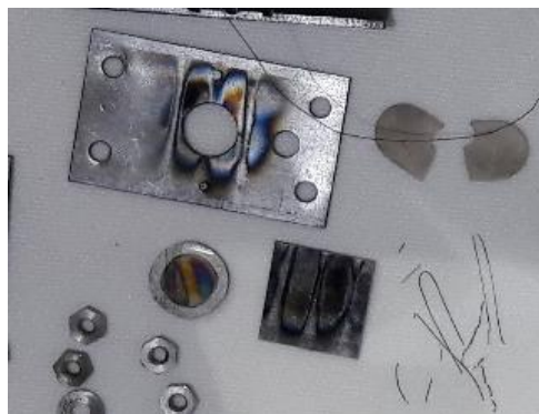
Figure 7.8. Zoom on the tungsten disk and tantalum plates. All the parts exposed to the filament show the same iridescent pattern on their surface and the filament broke at several places.
