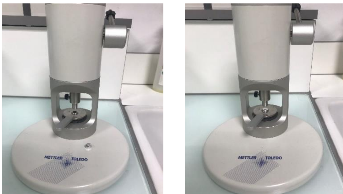
Figure 3.2.4.1. (left) Sealing press for Al crucibles for thermogravimetric analysis with Al cell and a cap (right) after the crucible was sealed.
