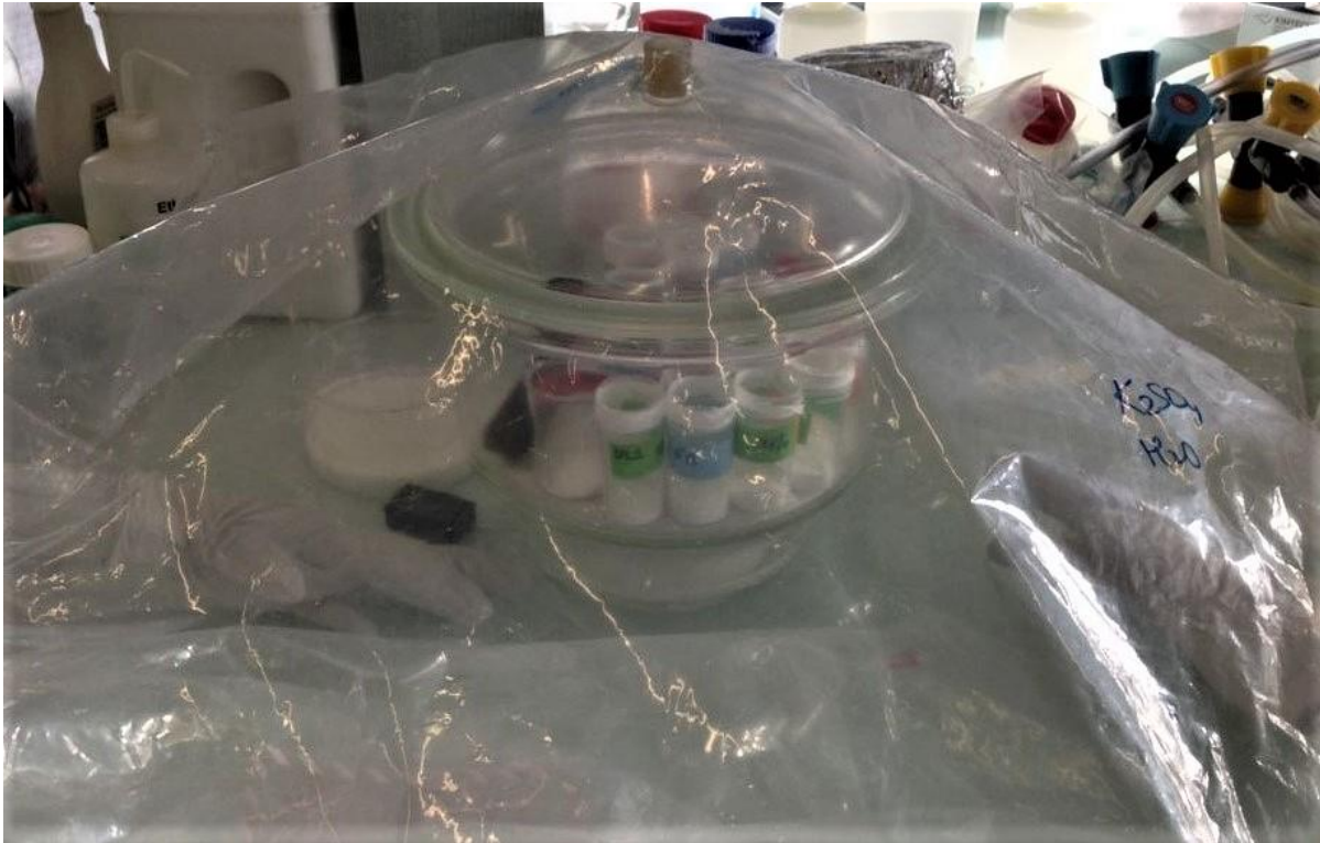
Figure 3.2.1.2. An example of C-(A)-S-H samples conditioned under certain RH atmosphere. The desiccator with a salt solution was put in the glove-bag with a salt solution. The hygrometers were kept inside the desiccators and the glove-bags to check the RH values.
