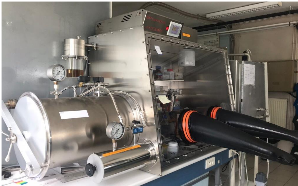
Figure 3.2.1.1. A wet glove-box used for synthesis, conditioning, and storing C-S-H samples at the geochemistry laboratory, ISTerre.
