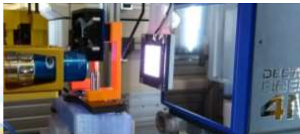
PolyPico on-demand droplet injector at VMXi, sample crosses beam \sim 100 \mu\text{s} , Eiger at 500 Hz (2 ms) 30 pL drop in calibration view
