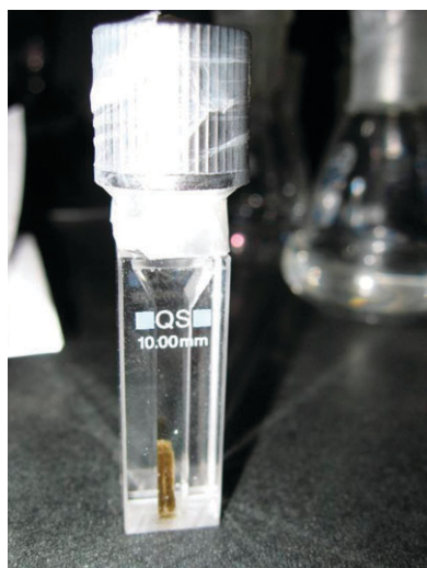
Fig. 2 Vermiculite clay gel in solution for measurement on D16.
