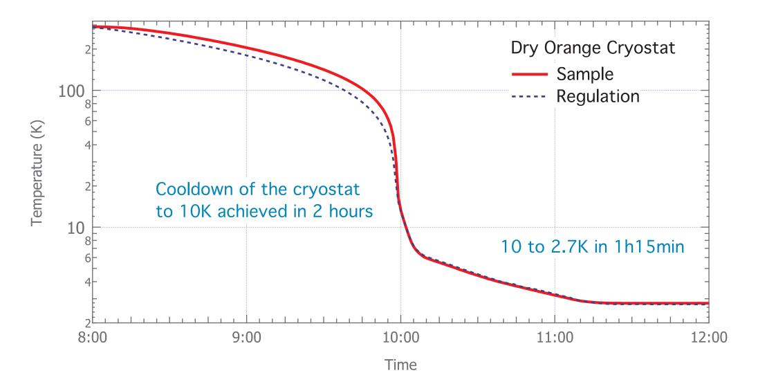
Once the compressor of the coldhead has started, it takes about 2 hours to reach 10 K at the sample.
