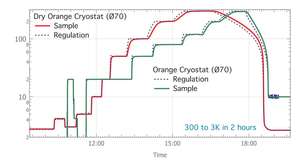
When carrying out an experiment, the performances of the dry cryostat are optimum if the user cool down the sample once and warm it up afterwards.
