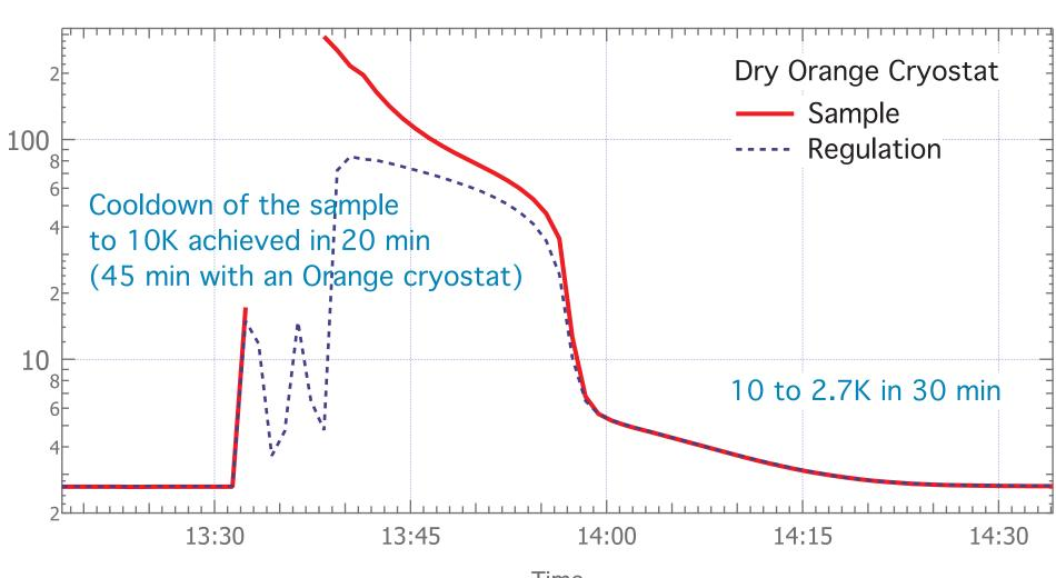
When the calorimeter is already at base temperature, 20 minutes suffice to cool down a sample to 10 K.
