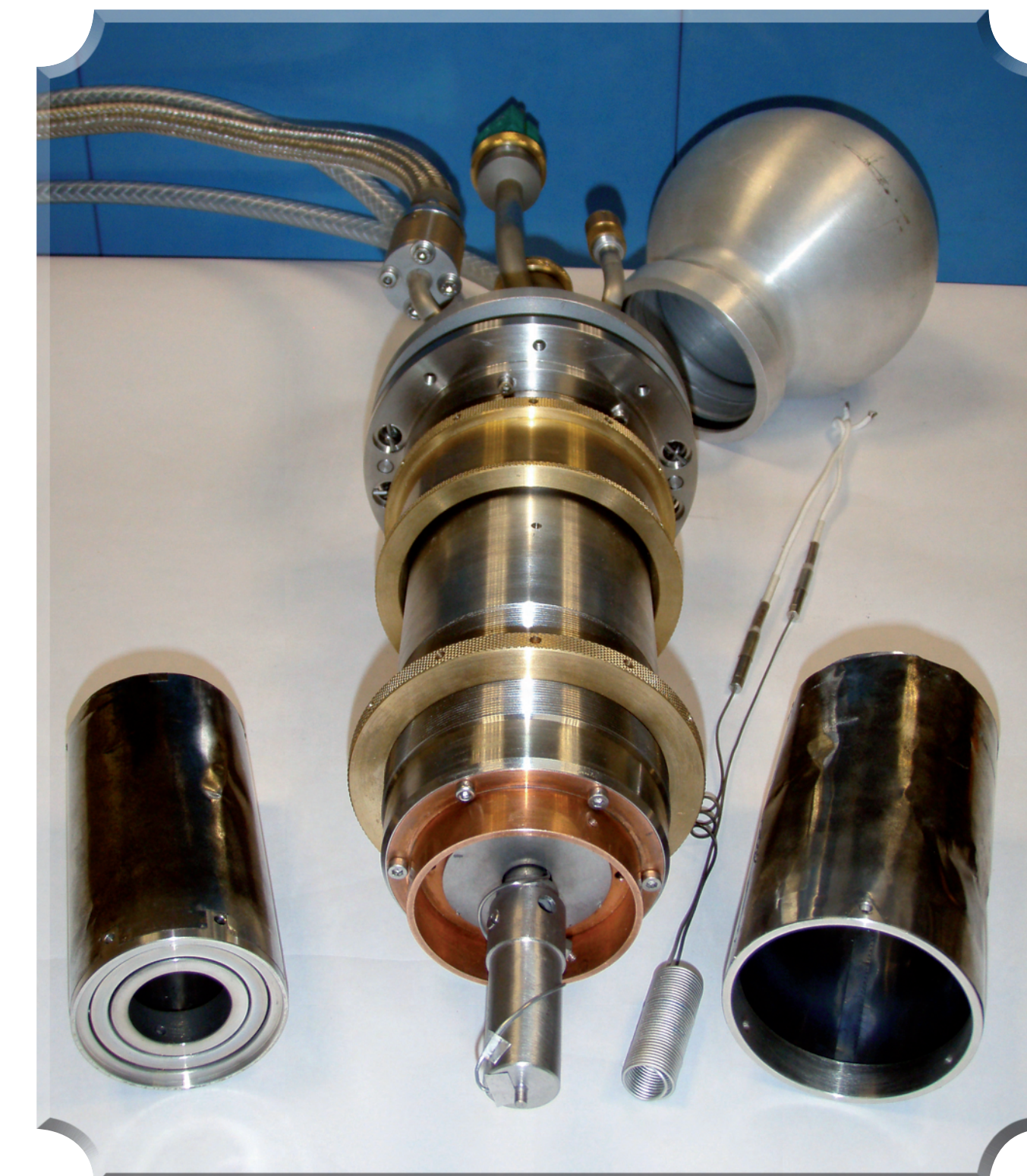
furnace with shields and spare heater apart
