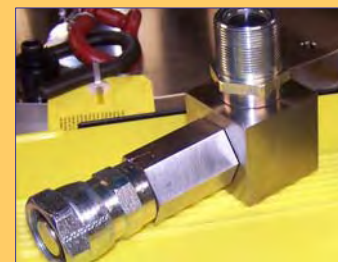
Long and short pin versions allow hoses to bypass each other at the 180 degree point for full 0 to 360 rotation.
