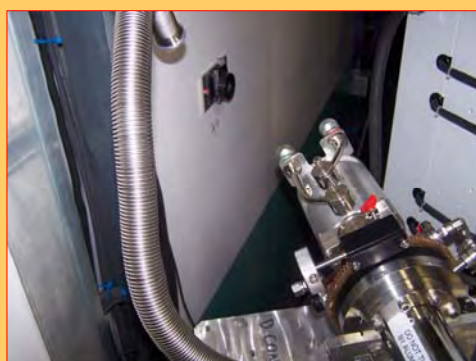
SNS CCR-11 (BL4a) is required to rotate 360 degrees on axis as well as 90 degrees perpendicular to the coldhead axis for sample changes.
