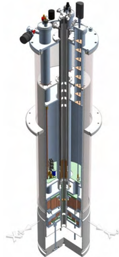
Cut-out view of the magnet (Courtesy Scientific Magnetics)
