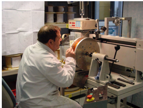
One of the 5T coils being wound.
