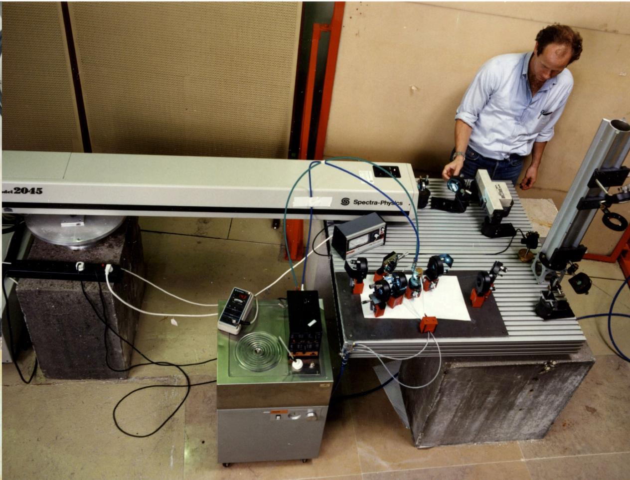
1990 - First test at ILL of a gaseous  $^3\text{He}$  neutron polarisation filter.
