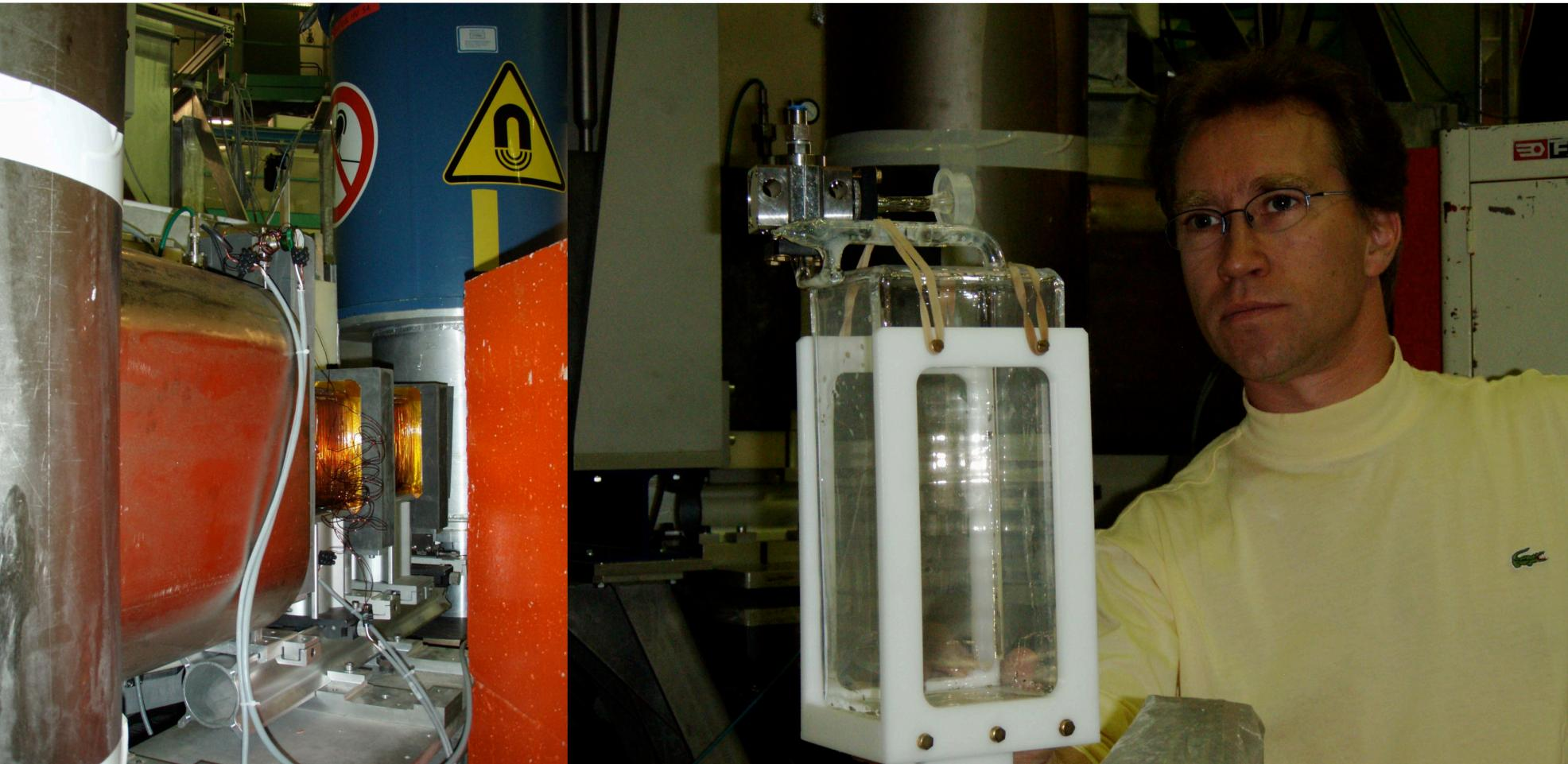
2008 - The new cryogen-free Cryopol is routinely used on D2o to investigate nanoscale samples. Eddy Lelièvre-Berna depolarises the world's biggest spin filter cell to calibrate the diffractometer.
