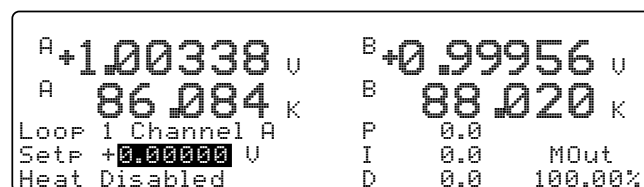
Normal Display with Temperature Setpoint Highlighted
