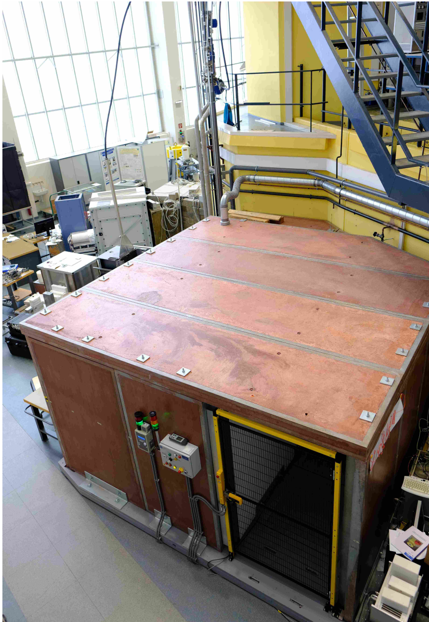
Fig. 1.4.: The shielding chamber of the new thermal white neutron beam facility at the TRIGA reactor. The chamber (red) has a size of \sim 5.2 \times 4.2 \times 2.2 \text{ m}^3 . The reactor (yellow) can be seen in the back. The entrance to the interior of the chamber is regulated by the mesh door which is part of a sophisticated interlock system. This allows access to the installed experimental setup at any time without requiring a reactor shutdown.
