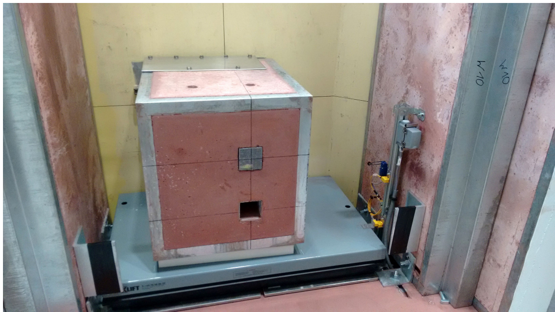
Fig. 3.6.: Open pre-chamber with installed shutter block ( \sim 70 \times 74 \times 67 \text{ cm}^3 ) standing on a hydraulic lift table. On the right the limit switches for positioning are visible. More pictures can be found in Appendix A.3.
