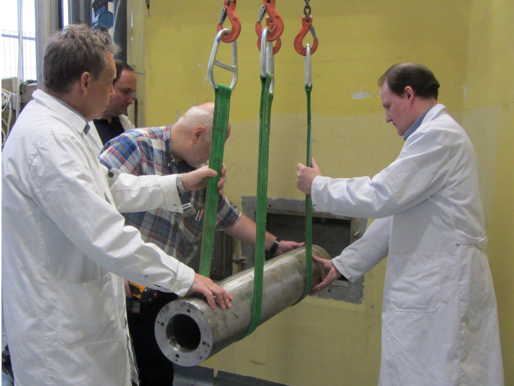
Fig. 4.14.: The beamtube insert right before installation. Dimensions to be found in Appendix A.4. Special thanks to Andreas Musilek, Mario Villa, Ernst Klapfer and Robert Bergmann (as seen from left to right)!
