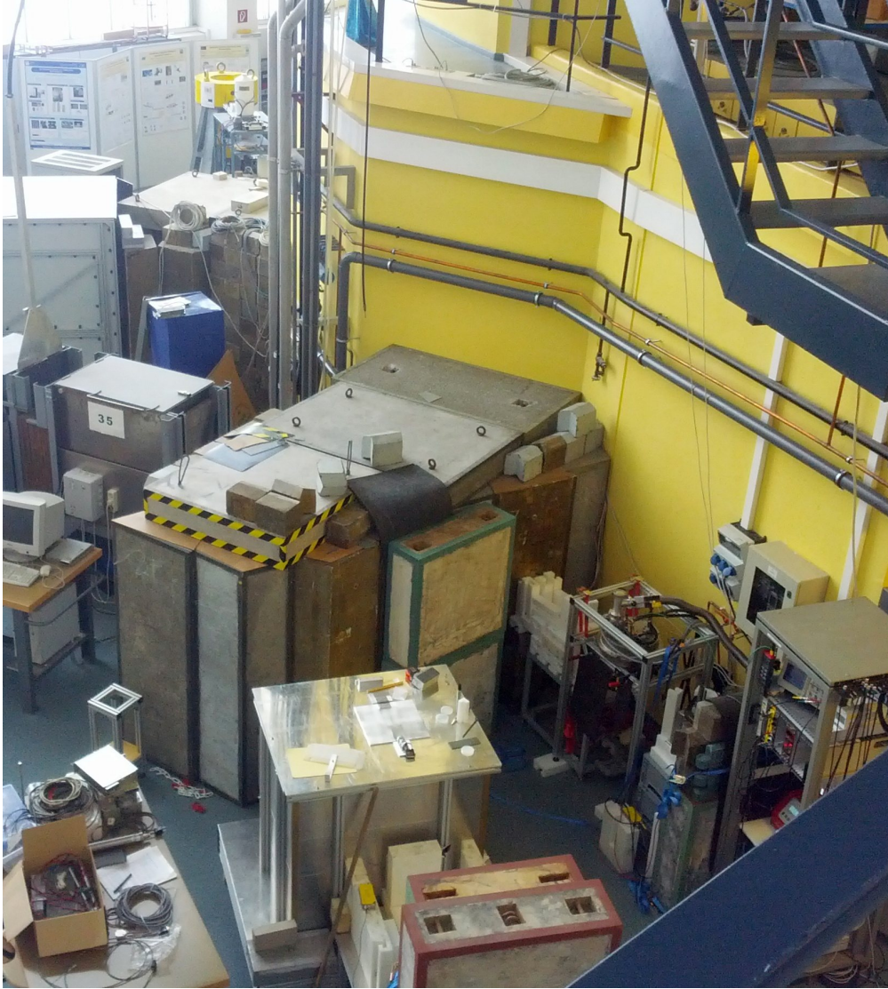
Fig. 1.3.: The beam line at the radial channel B of the TRIGA reactor in Vienna before the recent upgrade. A HOPG mosaic single crystal, mounted in front of the beamtube at the center of the heavyweight concrete radiation shielding, reflects a monochromatic beam out of the main beam. As it can be seen, its trajectory is almost parallel to the reactor wall. The components in the foreground are just residuals of a previous experimental setup.
