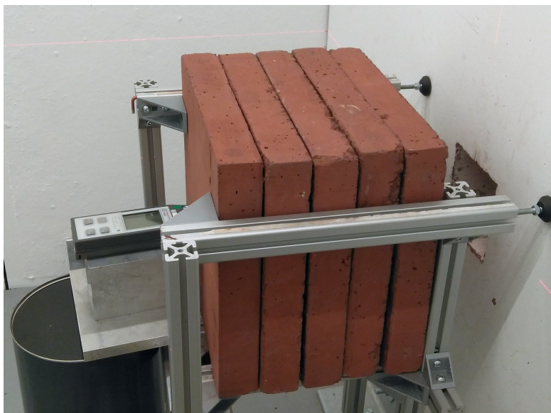
Fig. 4.1.: Measurement of dose rate and flux progression inside of shielding concrete slabs using the new neutron beam facility.
