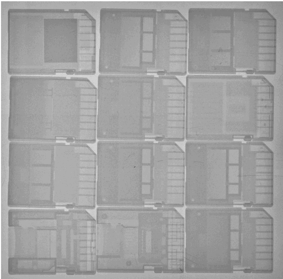
Fig. A.1.: Radiographic image of SD-cards and micro SD cards from different suppliers. It was taken at the Thermal White Beam by means a 2D-image plate detector. Exposure time: 60s. The image was taken for the IAEA to characterize SD cards.
