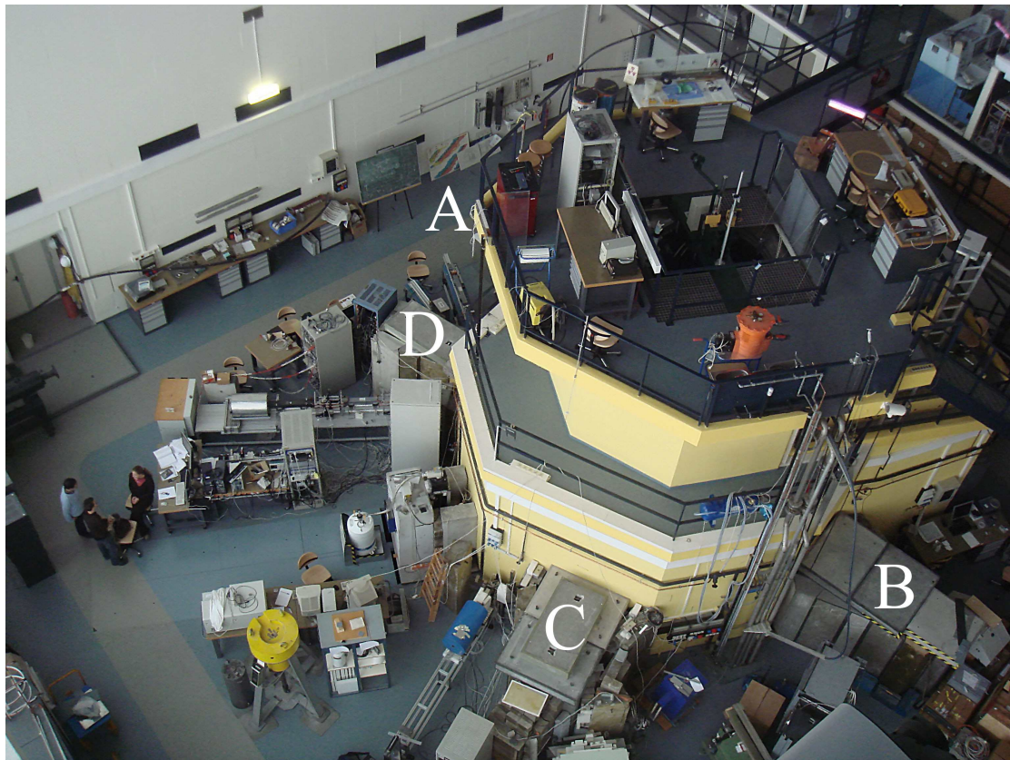
Fig. 1.2.: Massive heavyweight concrete blocks for radiation shielding are placed around the beam channels B, C, and D, where Bragg reflection at HOPG crystals is used to guide monochromatic beams through apertures of the radiation shields to the experimental setups. Between the channels C and D the radiography unit at the thermal column is seen, which is less demanding with respect to radiation protection. Right bottom corner: experimental installations at beam line B before the recent update.
